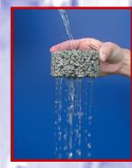
Permeable asphalt is another hard surface that will allow water to soak into the ground. It is extremely durable, can be plowed in the winter and will reduce ice buildup because water will not sit at the surface.
